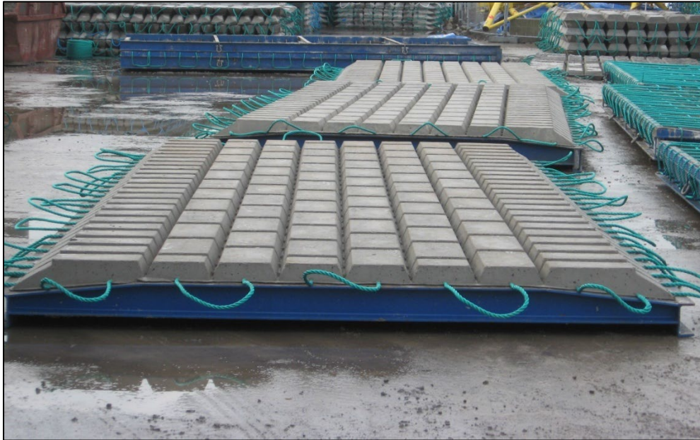
Figure 23: Example of Articulated Concrete Mattress
